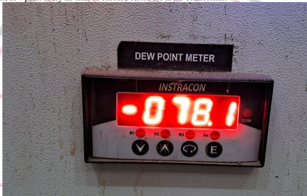
Fig. 4.1 Dew Point Measurement Display Showing Extremely Low Temperature
